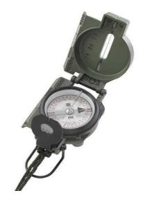
Graduated Azimuth (0-360°) in 5° units, the outer portion of the dial is graduated in mils. Sturdy aluminium case with metal hinges, painted olive green. Waterproof and shockproof. Build-in magnifying lens and 1:50,000 map scale die-cast on the side.
