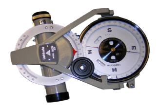
The Ushikata Surveying Compasses have been used for compass survey over the world for a long time. They are used for mountain, forest and land surveying work.
