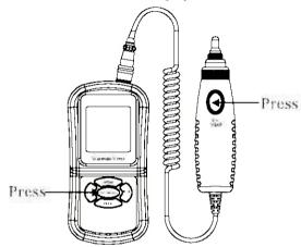
2. After the entire screen displays for 1 second, the default state is acceleration mode, if on the LCD displays the symbol or please promptly replace the battery, as shown in following figure:
