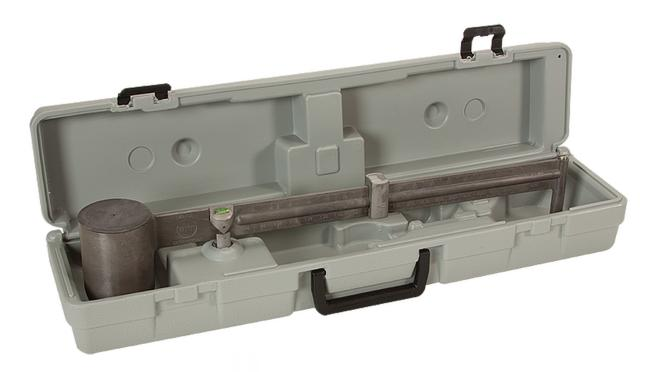
The Mud Balance provides a simple, practical method for the accurate determination of fluid density. The item's durable construction makes it ideal for field use. Despite its sensitivity, it contains no easily broken parts. Principally, the balance consists of a base and graduated arm with cup, lid, knife-edge, rider, built-in spirit level, and a counterweight. A plastic carrying case is provided to hold the balance intact and in it's working position.
