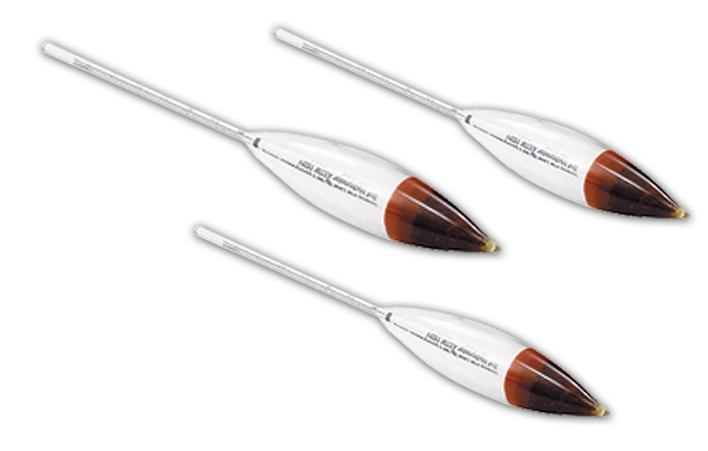
Soil Hydrometer A— H-4241
